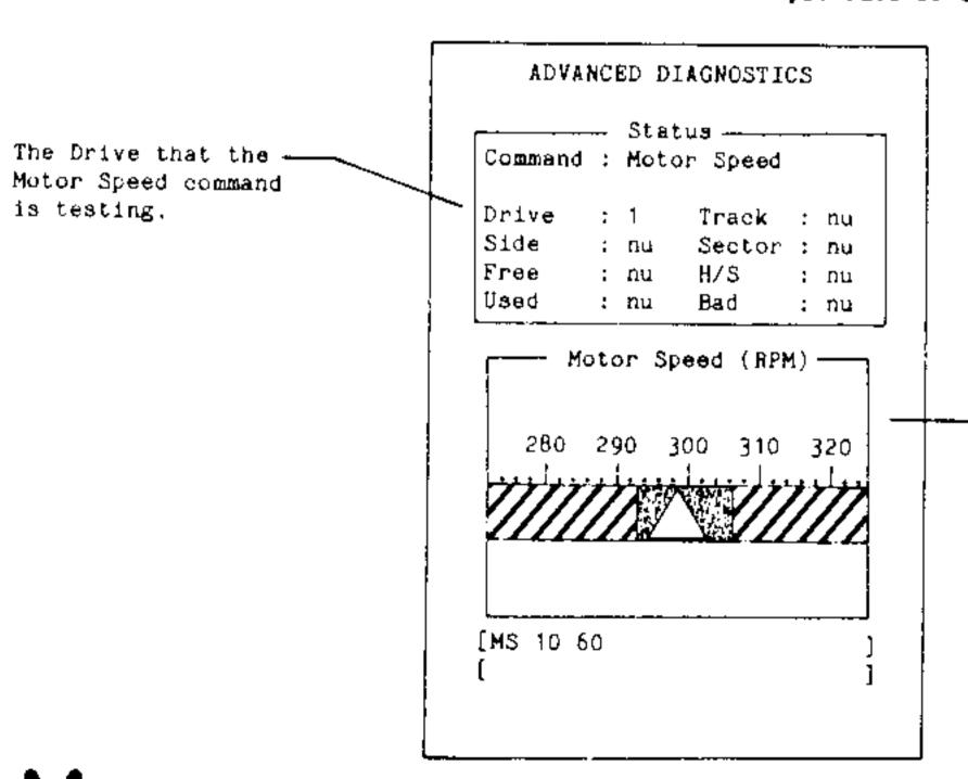
The Drives RPM is pointed to by the white arrow. If the point of the arrow stays in the Green area of the Bar, your drive is OK. If it is in the Red, your drive needs its Motor Speed adjusted to perform properly.
